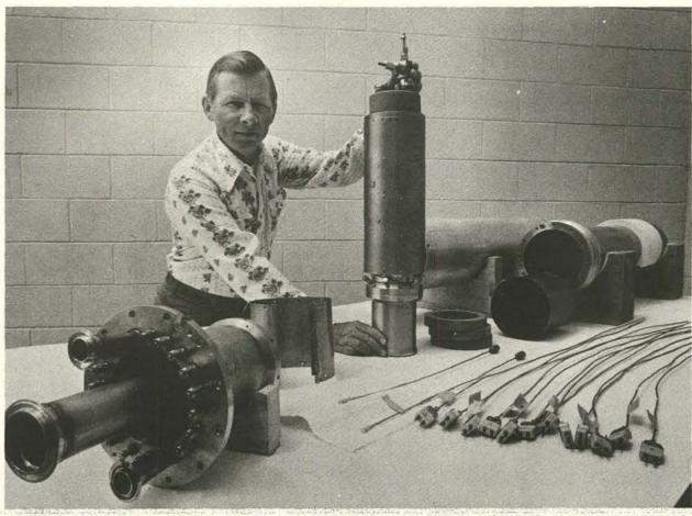
A TEST ASSEMBLY similar to this was used to simulate post-meltdown conditions in an LMFBR. The oxide fuel particles were in a can like the one in Joe Rivard's right hand. The rest of the capsule assembly is above the can. At left is the coolant assembly with ports for helium inlet and exhaust. At right are some of the thermocouples and pressure transducers used to instrument the experiment.
